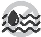
DO NOT install the indoor unit in a moist environment. Excessive moisture can corrode the equipment, electrical components, and cause electrical shorts.
