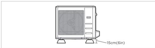
The outdoor unit must be installed on risers of at least 15cm(6in) in height or per local code to get unit above local mean snow fall.
