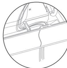
Replace foam gasket over wires.
