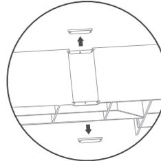
Remove knockouts as shown in the figure.
