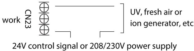
The WORK port is linked with the fan. When the fan is running, the relay is closed; if an active 24V signal is required, it can be directly connected to the G and C ports.
